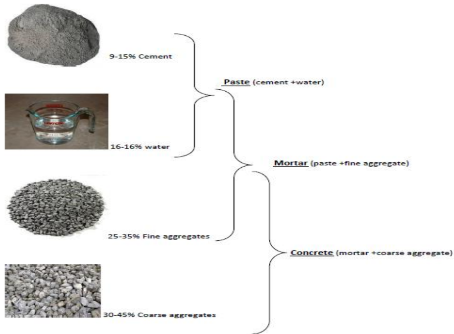
Figure 4: Percentage of concrete materials (values are depicted from www.concretenetwork.com )
