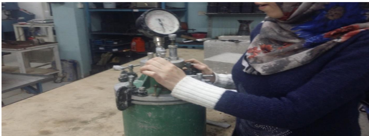
Figure 12: Air content test
