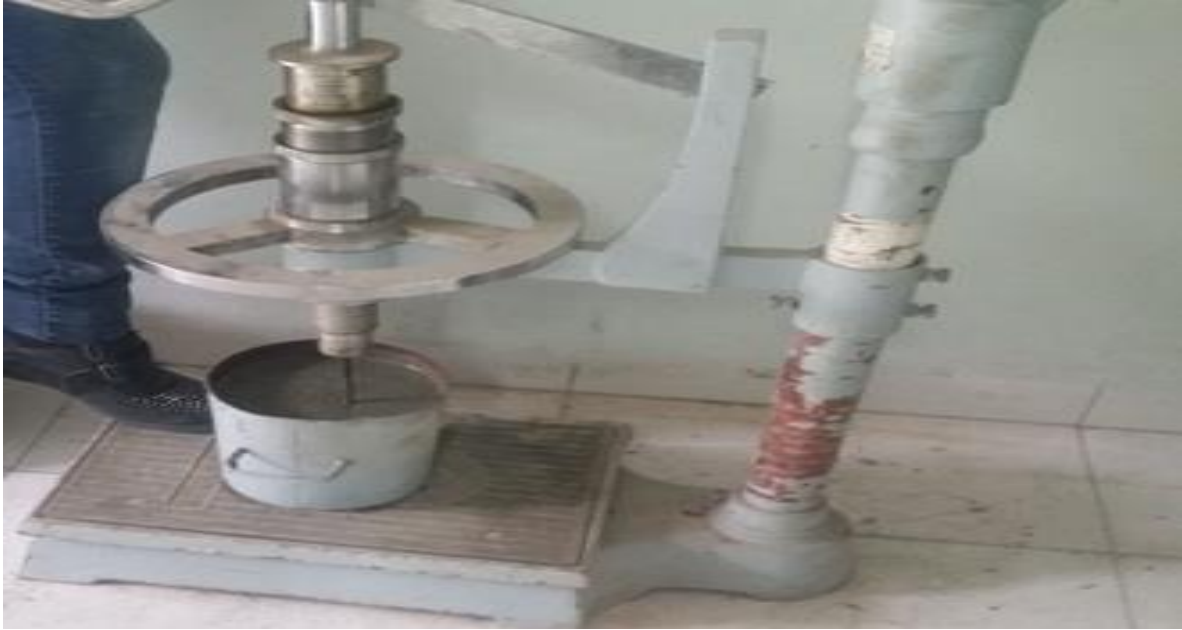
Figure 10: Concrete setting time test
